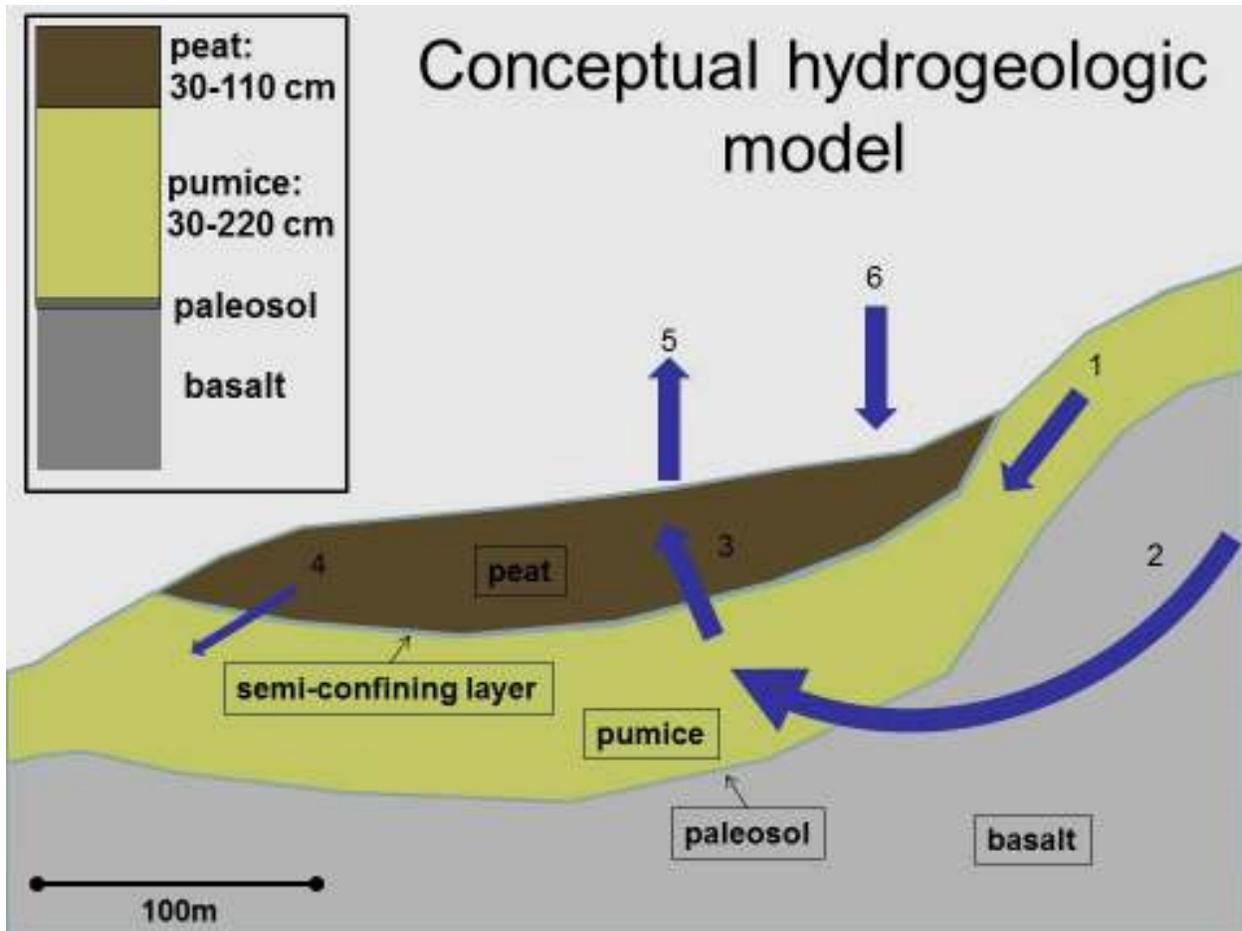
**Figure 5.** Conceptual hydrogeologic model cross section of the three study fens. Water balance elements are depicted as blue arrows: (1) shallow groundwater flow from local pumice deposits; (2) deeper groundwater flow through the basalt; (3) groundwater discharge from pumice to peat through leaky confining layer; (4) groundwater outflow from the fen to the pumice; (5) evapotranspiration; (6) direct precipitation.
