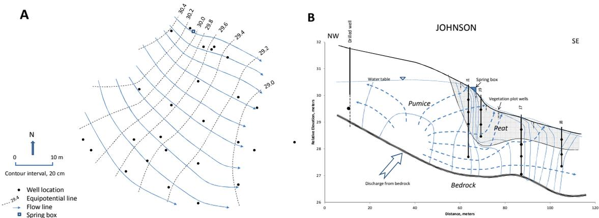
Figure 6. Flow nets generated to indicate flow of water through Johnson Fen based on water levels measured May 18, 2010. (A) plan view and (B) cross sectional view showing soils and geologic strata. Groundwater flow direction is indicated by flow lines (blue lines), and lines of equal hydraulic head (equipotential lines) are shown with dashed lines.
