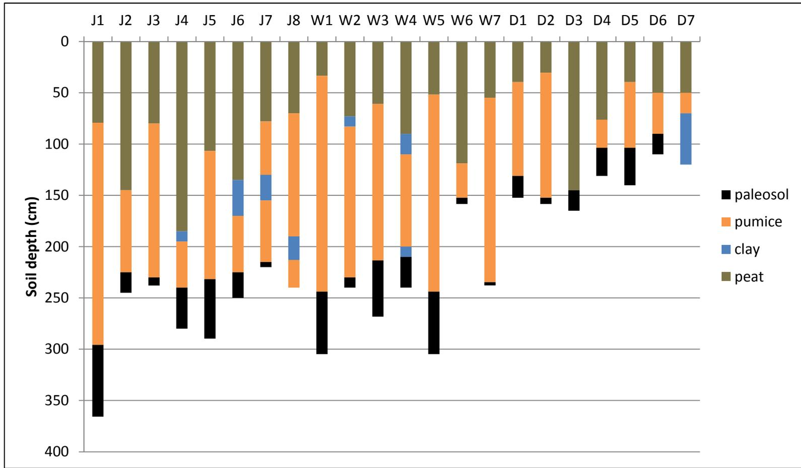
**Figure 3.** Soil profiles at well borings for the nested wetland piezometers, at Johnson (J1-J8), Wilshire (W1-W7), and Dry (D1-D7).
